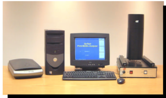
Print Mottle Analyzer and Paper PerFect Formation Analyzer sharing the same computer platform
