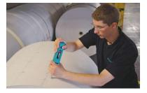
Intuitive operator interface (displaying hardness, profiles, limits, roll IDs, etc.).
