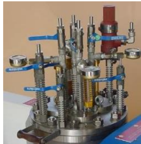
Detail of 4 chamber lid with optional thermometers and pressure gauges.
